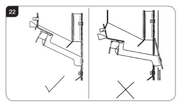
12.10 Replace the metal panel. There are spacers on the top edge to ensure the correct distance from the baffle. These interlock with the rear of the baffle, see Diagram 23.
