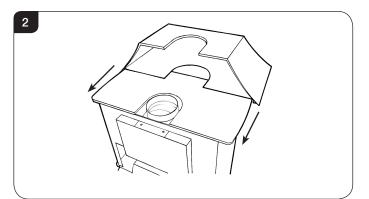
4.2 Make sure the appliance top fits into the guide along the bottom of the canopy, see Diagram 3.
