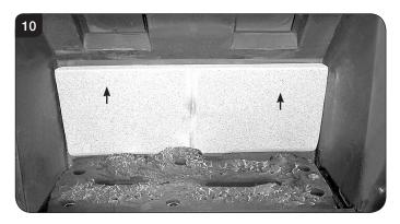
4.15 With the liners and baffle removed the firebox is clear for cleaning and maintenance, see Diagram 11.
