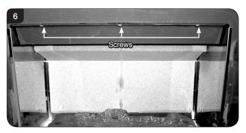
4.5 The baffle can now be removed through the front of the appliance.
