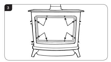
3.2 Lower the frame down to clear the top edge before lifting clear, see Diagram 4.
