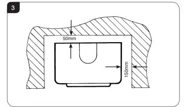
5.5 In a non-combustible recess be careful to allow enough clearance at the sides and rear of the appliance to perform spillage tests and reach the controls.
