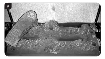
7.4 Place Log B on top of Log D. There is a hole on the underside of Log B which fits over the raised stud on Log D to secure in place. The right hand side of the log rests in the groove in the burner, see Diagram 10.
