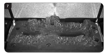
7.2 There are 3 embers. Place 2 embers in the back corners of the burner, resting in the cut outs, see Diagram 8. Place the last ember loosely at the front of the fuel bed to cover the hole in the centre.
