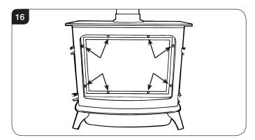
7.12 Replace ALL of the securing screws ensuring that a screw is present in all fixing slots.
