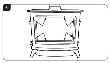
6.6 Lower the frame down to clear the top edge before lifting clear, see Diagram 7.
