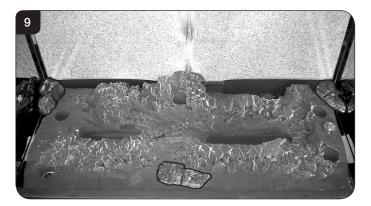
8.3 Place Log D on the left hand side of the burner. There is a hole on the underside of Log D which fits over the raised stud on the left of the burner. The back of the log should rest flat against the back panel, see Diagram 10.
