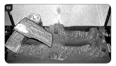
7.5 Place Log C on the right hand side of the burner. There is a hole on the underside of Log C which fits over the raised stud on the right of the burner. The back of the log should rest flush against the back panel, see Diagram 11.
