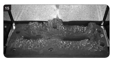
8.2 There are 3 embers. Place 2 embers in the back corners of the burner, resting in the cut outs, see Diagram 16. Place the last ember loosely at the front of the fuel bed to cover the hole in the centre.
