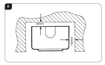
8.4 In a non-combustible recess be careful to allow enough clearance at the sides and rear of the appliance to perform spillage tests and reach the controls.
