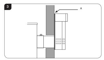
3.23 Feed the flue through the wall, making sure it runs smoothly.
