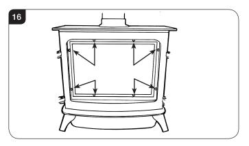
7.12 Replace ALL of the securing screws ensuring that a screw is present in all fixing slots.
