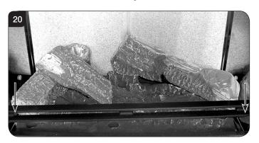
8.7 Place Log A across Log C. There is a hole on the underside of Log A which fits over the raised stud on Log C to secure in place. The small cut out on the left side of the log rests onto the log guard, see Diagram 21.
