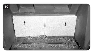
4.15 With the liners and baffle removed the firebox is clear for cleaning and maintenance, see Diagram 11.
