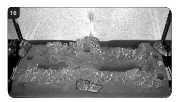
Place Log D on the left hand side of the burner. There is a hole on the underside of Log D which fits over the raised stud on the left of the burner. The back of the log should rest flat against the back panel, see Diagram 17.
