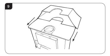
4.2 Make sure the appliance top fits into the guide along the bottom of the canopy, see Diagram 10.
