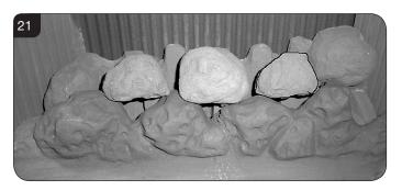
8.17 Place the rear left medium coal on the recess behind the front row of coals resting on the rear panel, Diagram 22.
