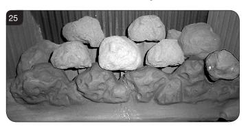
5.20 Place the left hand small coal in the recess between the flame baffle and the front coal, Diagram 26.
