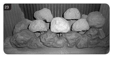
8.19 Place the right hand small coal in the recess between the flame baffle and the front coal, Diagram 24.
