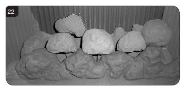
8.18 Place the rear right medium coal in the recess behind the front row of coals resting on the rear pane, Diagram 23.
