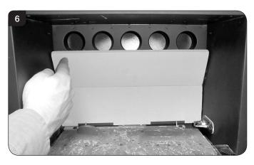
When refitting the top liner rear liner, ensure that the chamfer is placed downwards.
