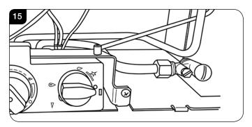
6.2 Connect a suitable pressure gauge to the test point located on the inlet fitting and turn the gas supply on. Light the appliance and check all gas joints for possible leaks. Turn the appliance to maximum and check that the supply pressure is as stated on the databadge. Turn the gas off and replace the test point screw, turn the gas on and check the test point for leaks.
