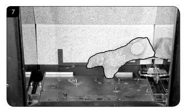
7.3 Place Log B over the two middle studs on the burner tray, see Diagram 8.
