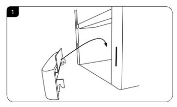
2.2 Remove the frame to gain complete access to the control valve and the viewing aperture by lifting the hooks clear of the slots on the front of the appliance, see Diagram 2.
