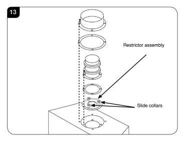
5.48 Flue Lengths over 5m (CL5 Top Exit) and Flue Lengths over 6m (CL8 NG)
