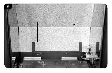
4.5 Slide the lower rear liner up and out of the lower bracket, see Diagram 6.
