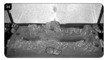
9.19 Place Log D on the left hand side of the burner. There is a hole on the underside of Log D which fits over the raised stud on the left of the burner. The back of the log should rest flat against the back panel, see Diagram 35.
