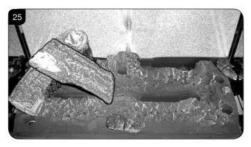
7.21 Place Log C on the right hand side of the burner. There is a hole on the underside of Log C which fits over the raised stud on the right of the burner. The back of the log should rest flush against the back panel, see Diagram 26.
