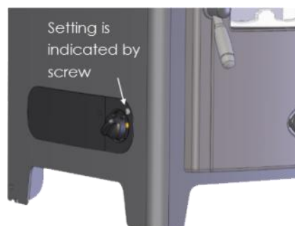
Figure 1: Setting the thermostat
