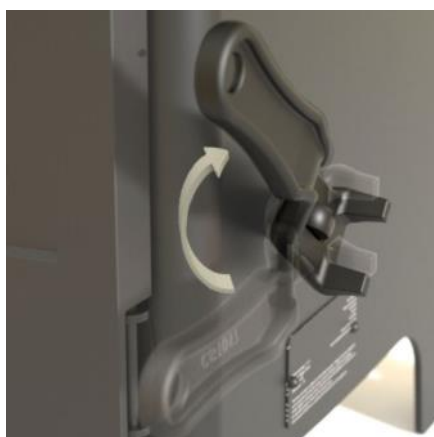
Figure 4 Use the operating tool on the riddle control
