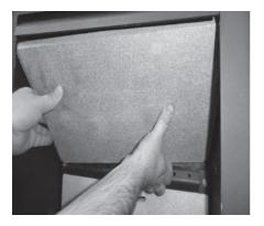
Remove the upper secondary steel baffle and internal vermiculite baffle (for further instruction please see under maintenance heading).
