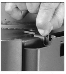
Remove both cotter pins from the retaining bar
