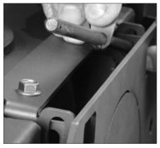
Remove the retaining bar by sliding it in any direction and angling the bar upwards before sliding the bar fully out of the brackets
