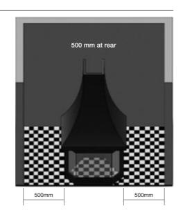
500mm at each side and 500mm at the rear of the appliance from any combustible materials. If using single wall flue pipe, there must be a clearance of at least 3 times the diameter of the flue pipe (e.g. 125mm diameter pipe = 375mm minimum clearance) from any combustible materials e.g. wooden beam.
