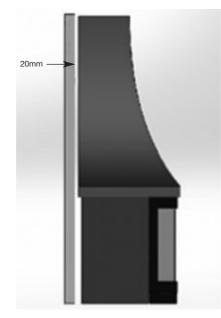
6 Install the canopy onto the top support bracket and position the canopy ensuring that there is a minimum 20mm air gap between the rear of the canopy and the noncombustible wall, once in position drill and self-tap the underside of the canopy through the top support bracket
